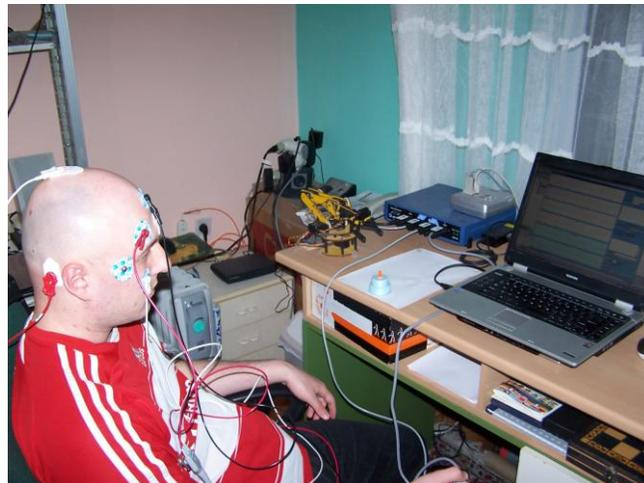
Figure 6. Experimental setup: subject, electrodes, robotic arm, biopotential amplifier, two disk Tower of Hanoi, and computer.
