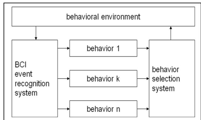
Figure 4. The BRI approach using behavior based robot control architecture
