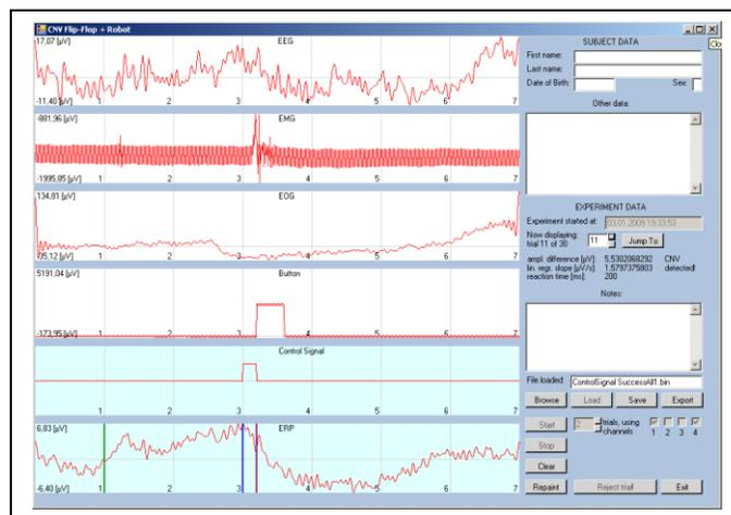
Figure 7. An experimental trial with CNV control of behavior-based robotics
